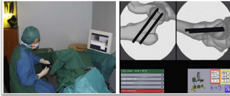
Figure 6. The hip fracture surgery simulator system replicates a real surgical environment (left) and the visual feedback is provided through simulated fluoroscopy images (right).
