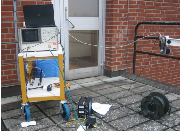
Figure 3.7: An HP 8720C VNA was used in the channel measurements with the virtual linear array. In the photo, on top of the VNA a laptop with Labview was used to control the measurement.
