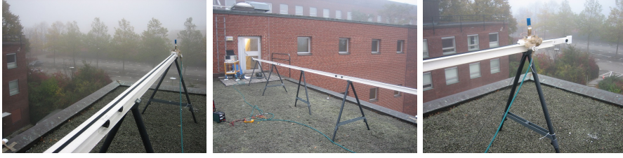
Figure 3.5: Photos of the virtual linear array used during a measurement. An omni-directional antenna moves on a rail, and measures the channel at 128 equidistant positions with half-wavelength spacing at 2.6 GHz. This yields a large array that spans 7.4 m in one dimension.
