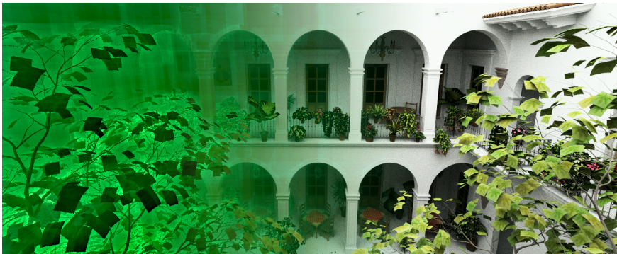
Figure 1: The San-Miguel scene (7,842,744 triangles) overlaid with a visualization of its Bonsai bounding volume hierarchy (BVH). The Bonsai BVH of San-Miguel is constructed in 478 ms using a 2.6G Hz quad core laptop CPU (Intel 4950HQ) and rendering performance is 107% compared to the rendering performance of the same scene using a BVH built with the sweep SAH method.
