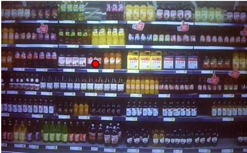
Figure 3.6: Data point from a mobile eye-tracker that is mapped onto the scene video. Here the gaze is indicated with a red dot.
