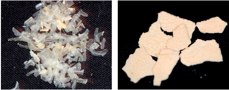
Figure 3 Image showing the low-temperature, protein-rich fouling produced in the pre-heating section (left panel). This fouling type is thin and translucent, whereas the mineral-rich UHT fouling (right panel) is thicker and has a rough surface.
