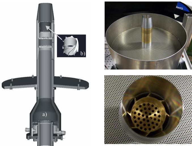
*Figure 2.13 A cross-section of the low-swirl burner is shown at the left. A photograph of the burner and the co-flow surrounding it is shown at the upper right and a photograph of the inside of the burner nozzle is shown at the lower right, the vanes and the perforated plate being visible.*
