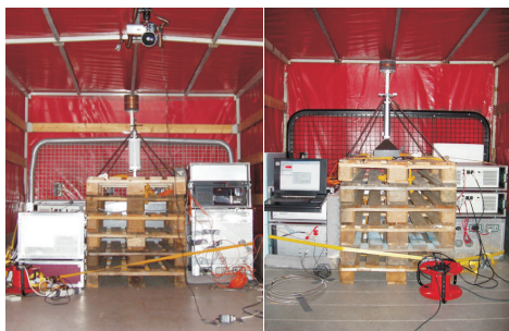
Figure 4: Loading spaces with the measurement equipment — left Rx, right Tx
