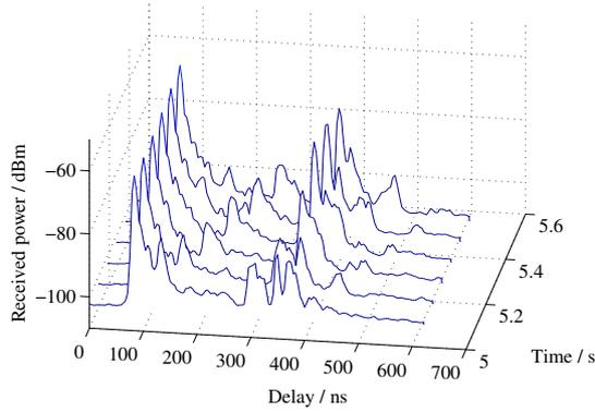
Fig. 7. Short-time average PDPs from 5 s to 5.5 s
