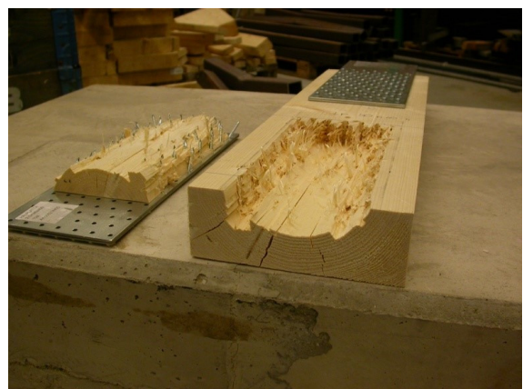
Figure 1: Nailed steel plate connection loaded in tension (a), plug shear failure (b) and specimen after experimental test (c)
