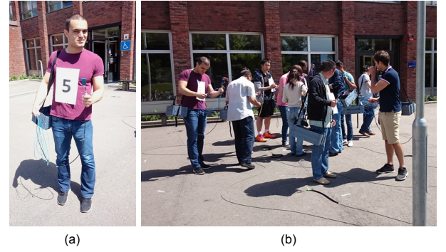
Fig. 2. (a) A user holding the MS user equipment antenna with an inclination of 45°. (b) Users moving randomly within the five-meter diameter circle at UE site MS 4.
