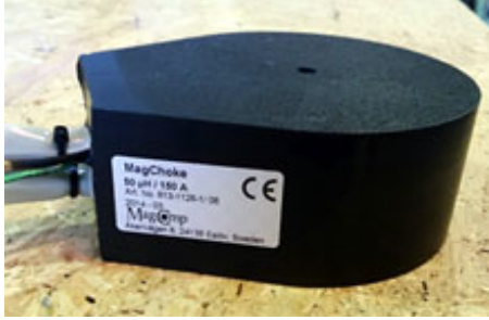
Figure 57: MagChoke, 50 \mu\text{H} , 150 A, 118 mm diameter, 52 mm height.
