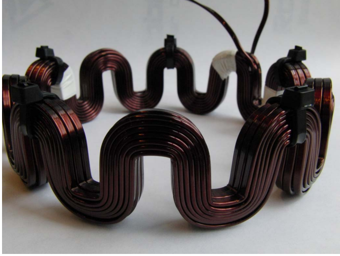
Figure 36: Wave winding with 35 mm press height [55].
