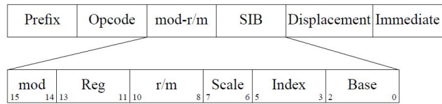
Figure 4.1: Illustration of a x86 instruction
