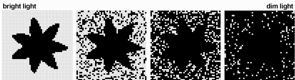
Fig. 2 The effect of photon shot noise.
