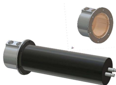
Fig. 1. The NE-213 detector. Top: the scintillator “cup”. The optical boundary is provided by a borosilicate-glass window (light brown). Bottom: The gray cylinder to the left is the “cup”. The black cylinder to the right is the  $\mu$ -metal shielded PMT and base assembly. Figure from Ref. [6]. (For interpretation of the references to color in this figure caption, the reader is referred to the web version of this article.)
