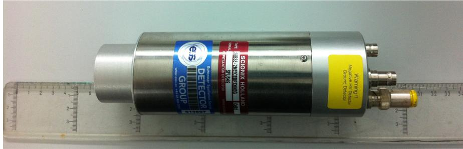
Figure 2.4: Photograph of the  $\text{CeBr}_3$  detector. The scintillator crystal is to the left. The PMT and the base are to the right.
