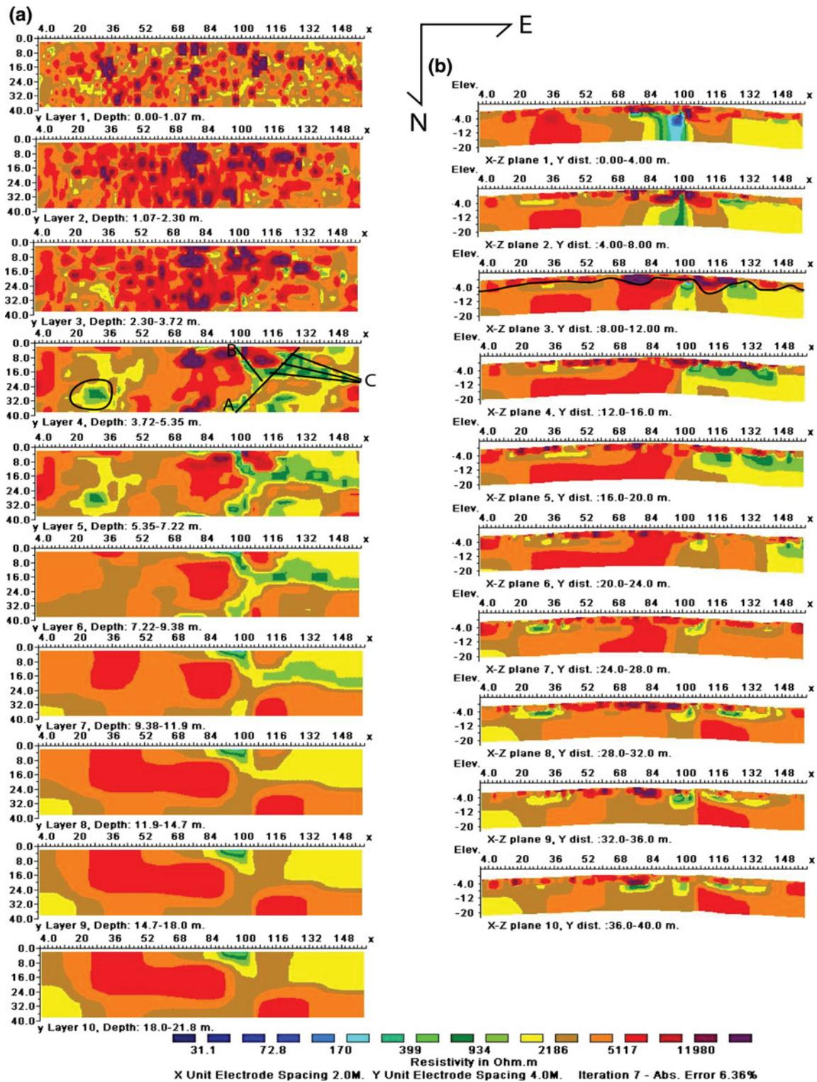
**Fig. 11** Bäckседа Electrical Resistivity Imaging from 3D inversion, direction indicator shown at the top; **a** horizontal slices, ERIH, interpretation of weakness zones/anomalies are added to graph four
