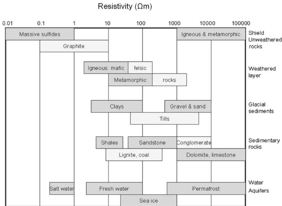
lower the resistivity. Massive sulphides and graphite are very conductive and have resistivity values below 10 Ωm (Fig. 6). Graphite is often the connecting link in mineral zones (Telford et al. 1990).
