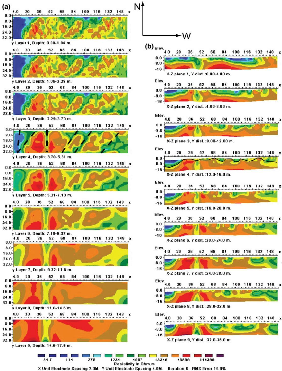
**Fig. 10** Olunda electrical resistivity imaging from 3D inversion, direction indicator shown at the top; **a** horizontal slices, ERIH, interpretation of weakness zones are added to graph four from the top;
