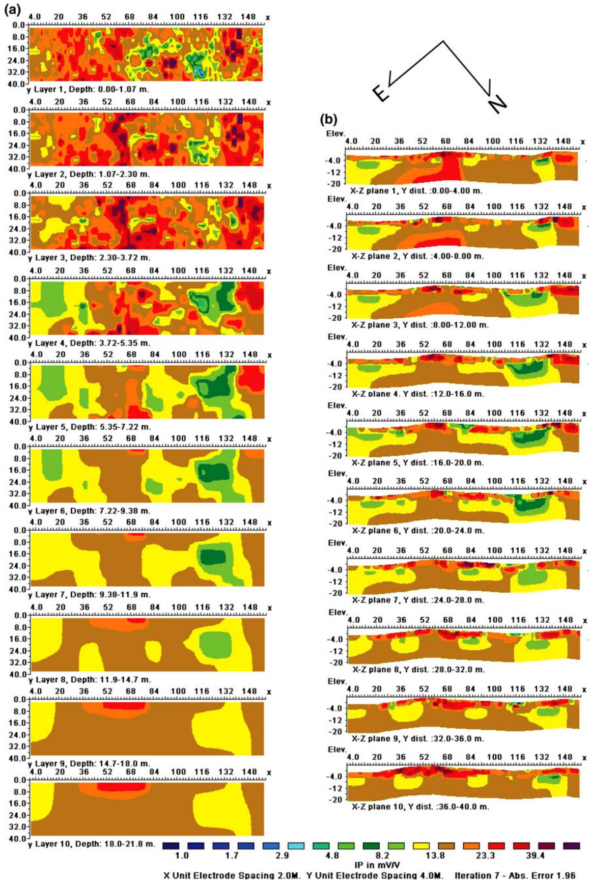
◀ **Fig. 15** Dalby-induced polarization from 3D inversion, direction indicator shown at the top; **a** horizontal slices, IPH; **b** vertical slices, IPV
