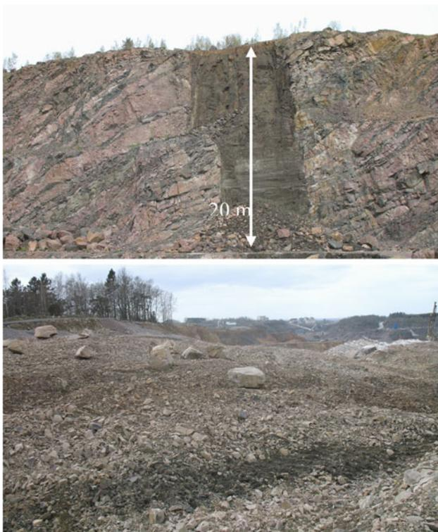
**Fig. 4** Top quarry face at Dalby, note the diabase dyke in the middle, bottom surface at Dalby, after removal of the overburden
