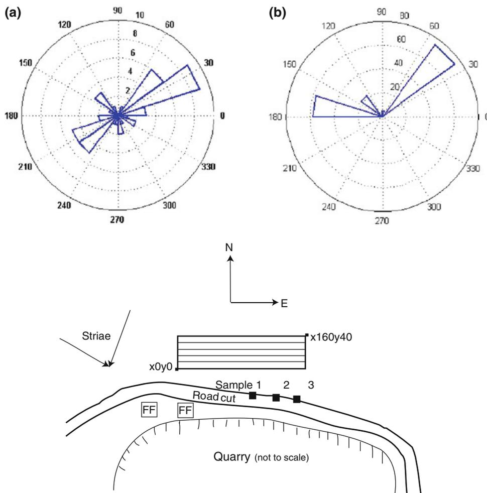
rock mass, close to the face of the quarry, in the area that had been cleared from overburden. The length and trend of fractures in 100 m<sup>2</sup> areas was established. The total length of all the fractures divided by the area gives an index value for the fracture frequency, FF Index.
