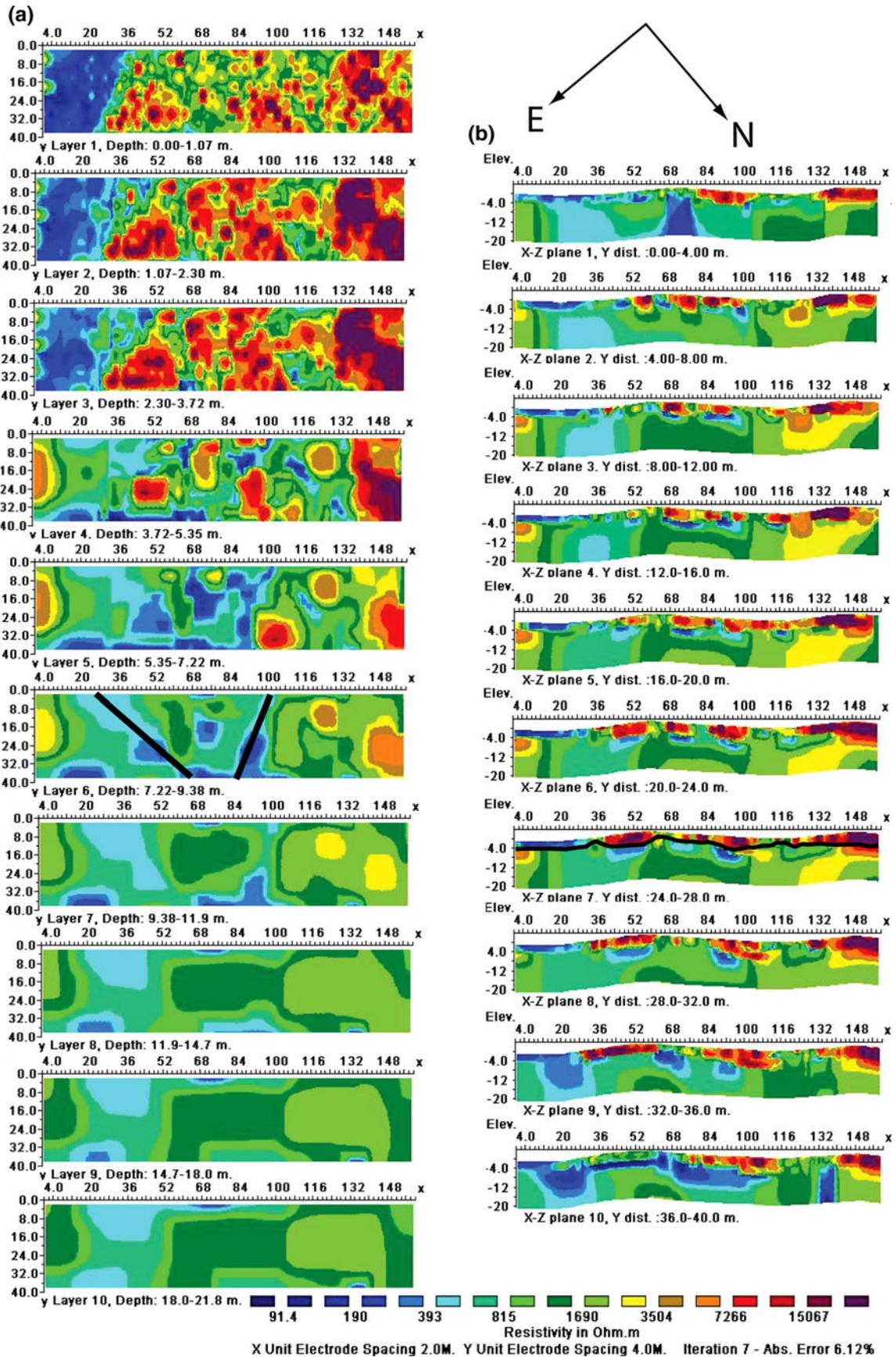
◀ **Fig. 14** Dalby electrical resistivity imaging from 3D inversion, direction indicator shown at the top; **a** horizontal slices, ERIH, interpretation of weakness zones/anomalies are added to graph six from the top; **b** vertical slices, ERIV, two different interpretations of the thickness of the overburden is added to graph seven from the top
