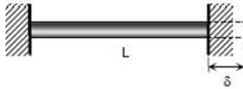
Fig. 4.1 Bar with both ends fixed [75]
