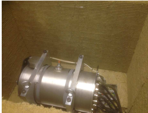
Fig. 6.13 EM3 placed inside a temperature insulated chamber [107]
