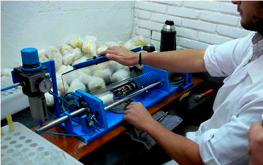
Figure 6.8 Air-flow cutter. Diminutive samples are cut out with an air-flow apparatus and inserted into tiny test tubes
