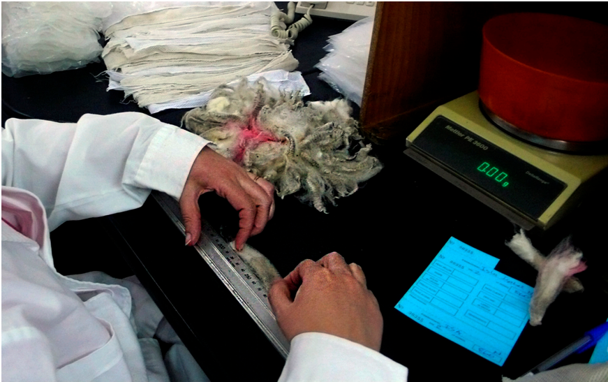
Figure 6.7 Measuring the length of the samples.
