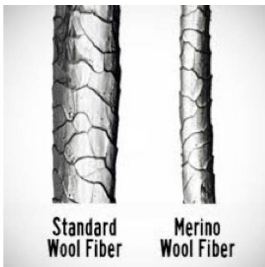
Figure 6.11 Close up comparison between Merino wool fibre and other wool fibre.
