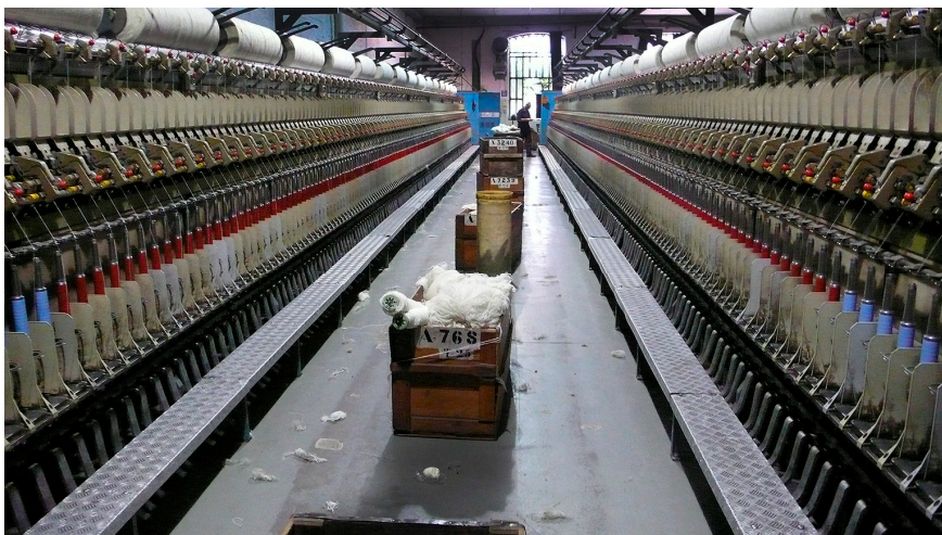
Figure 7.8 Industrial spinning machine.
