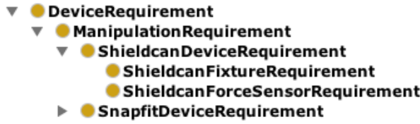
Figure 11: The device requirements of the skill ShieldCanInsertion are modelled in an ontology. The ManipulationRequirement which several skills inherit from, is that a gripper has to be mounted on the robot. The ShieldcanFixtureRequirement and the ShieldcanForceSensorRequirement list that there must exist a fixture and a force sensor that have to be vertically aligned (not shown in the picture).
