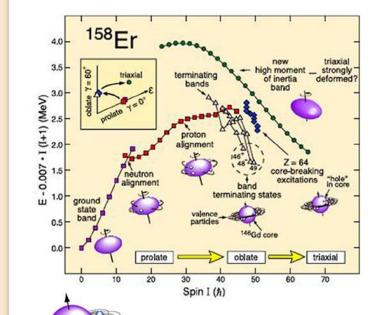
The nucleus of <sup>158</sup>Er exhibits different shapes as the frequency of rotation (spin) encreases (x-axis) with increasing spin, the shape changes from prolate (like a cigar) to oblate (like a pancake), and finally becomes triaxial (the three axes are different). When the shape of the nucleus is oblate, terminated band behaviour is seen, where the energy of the system (y-axis) varies irregularly.
