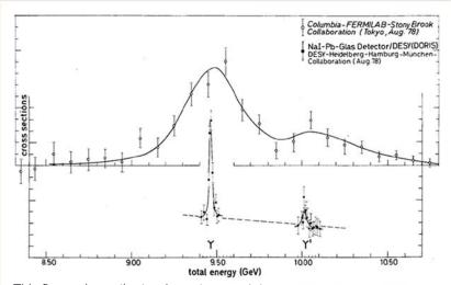
This figure shows the two lowest mass states of the Y particle, and illustrates the difference in resolution between a proton accelerator (above) and an electron-positron collider (below).
