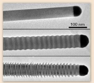
Nanowires with and without a heterogeneous structure.
