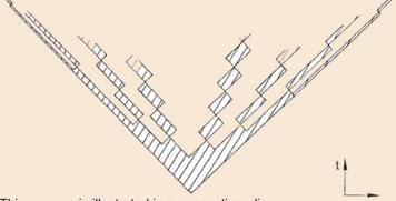
This process is illustrated in a space-time diagram, in which time extends upwards. The extension of the force field is shown by the hatched area.
