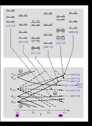
The lower figure shows the Nilsson diagram for Z = 50-82. In the deformed nuclei, the axis of symmetry is about 30 % longer than the orthogonal axis, with corresponding values of  $\varepsilon = 0.25 - 0.30$ .
