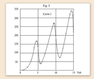
The experiment showed that electrons accelerated through mercury vapour are slowed down when the electrons reach a certain amount of energy, which confirms that an atom can only take up energy in quantised steps.
