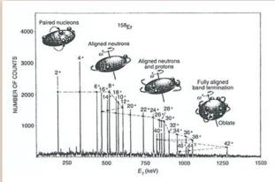
Energies of γ-rays emitted when excited rapidly rotating nuclei decay, with illustrations showing how the angular momentum is developed in different phases.
