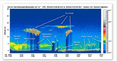
Vertical profile of the atmosphere obtained using lidar (laser radar) on the satellite CALIPSO. Both hot (water) and cold (ice) clouds are formed on the aerosol particles.
