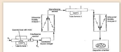
Illustration of the aerosol generation system in which nanoparticles with a narrow size distribution are made and deposited in a controlled way onto a substrate.
