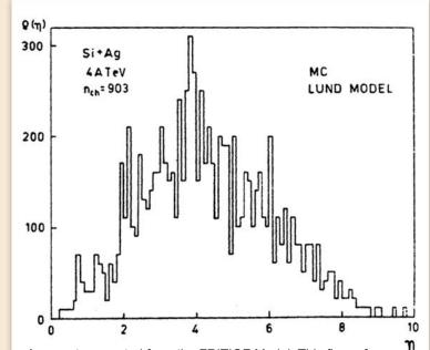
An event generated from the FRITIOF Model. This figure from 1986 shows the distribution of particles in a high energy collision between a silicon and a gold nucleus.
