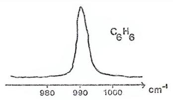
A figure from Aldén's Master's project, which was the first step towards combustion physics in Lund, showing a coherent anti-Stokes Raman spectroscopy (CARS) spectrum of benzene, recorded at 1.30 a.m. on 23<sup>rd</sup> December 1977. This turned out to be an important part of his study.
