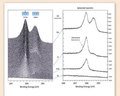
The 1s carbon peak indicates binding of CO on the surface of the material. The figure on the right shows more detailed spectra that reveal vibrational levels.
