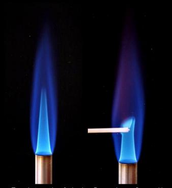
Two photographs of a laminar Bunsen burner flame, without a probe (left) and with a thermo-element inserted into the flame (right) to measure the temperature at a specific point. Insertion of the probe leads to changes in the flow, causing a lowering of the temperature and changes in the chemical reactions taking place. This can be avoided by using non-intrusive laser diagnostics.
