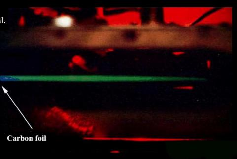
A beam of lithium ions passes through a thin carbon foil, allowing two atomic decays to be observed, one which is short-lived (5 ns), and can be seen as the blue light, and a longer-lived one (46 ns), seen as the longer-wavelength green light.
