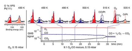
The experiment reveales a new carbon dioxide gas phase peak at temperatures around 535 K.
