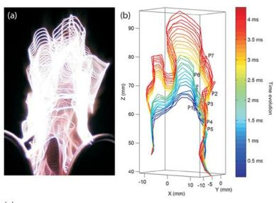
(a) Photograph of a sliding discharge plasma. Like our own eyes, a normal camera cannot discern the discharge as it moves rapidly in the air flow.
