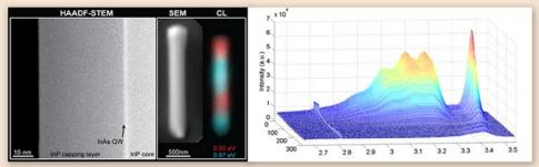
Photoluminiscence. This method gives high spectral resolution for the optical characterisation of semi-conductor materials.
