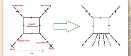
First-order diagram with an incoming real photon, which is split into a virtual electron-positron pair, which in turn couples to the core via virtual photons at the points marked X. In the final state a real photon is recreated.
