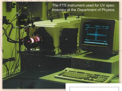
FTS gives very high resolution, allowing the structure of spectral lines resulting from the spin of the atomic nucleus to be seen.
