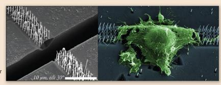
Hollow nanowires for the injection of cells.
