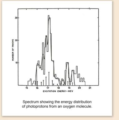
The oxygen nucleus (16O) was irradiated with gamma rays from the synchrotron, causing it to become excited. Protons were emitted from the excited nucleus, and detected by the tracks made in photographic emulsions. The energies of the protons could then be determined from these tracks.
