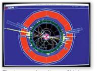
Electrons and positrons of high energy are collided in the Large Electron-Positron collider (LEP) at CERN. This leads to the formation of a quark, an antiquark and a large number of gluons. The production of these multigluon states is well described by the dipole formulation. which is simulated in the Monte Carlo program ARIADNE.
