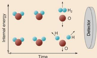
This example shows how the geometry of a water molecule is changed by electron decay which affects the molecular orbitals creates bonds between the atoms.
