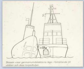
Explanatory sketch of the positioning of the detector as close to the submarine as possible. The long horizontal tube pointing towards the submarine contains the sensitive gamma detector.
