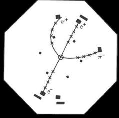
Tracks from a J/psi meson, which decays to two pions (pi $^+$ , pi $^-$ ), an electron (e $^-$ ) and a positron (e $^+$ ). The J/psi meson consists of a charm quark and its antiquark.
