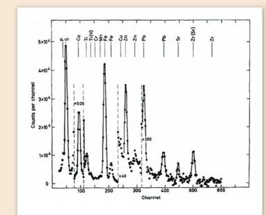
The spectrum obtained from matter deposited on a carbon foil left outdoors for one day shows the presence of significant amounts of sulphur and calcium, as well as zinc and lead, in the air we breath. Both K and L X-rays can be seen.
