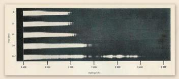
Solar spectrum observed at increasing height with the first rocketborne spectrograph. In the bottom spectrogram the rocket has passed through the ozone layer 50 km above the earth's surface, and for the first time one can see a part of the Sun's ultraviolet spectrum.
