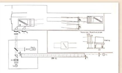
$S_{A}$ Entrance-slit for the lens equipment Immersion-grating in autocollimation Α
