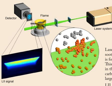
Illustration of the measurement of soot concentration (volume fraction) in a laboratory flame.
