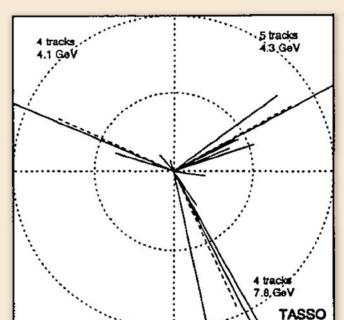
Figure from the TASSO experiment at DESY in Hamburg, which demonstrated the existence of gluons, thereby confirming the theory of QCD. The figure shows three particle showers from a quark, an antiquark and a gluon created by the collision between an electron and a positron.
