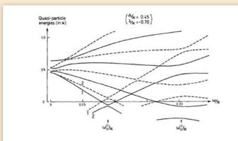
Energy levels in nuclei as a function of the rotational frequency of the nucleons, according to the Bengtsson-Frauendorf-formalismen. At the two frequencies indicated on the x-axis, the energy levels interact, giving rise to so-called backbending.
