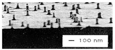
Scanning electron microscopy image showing freestanding columns of indium phosphide after an indium phosphide surface covered with silver particles has been etched.
