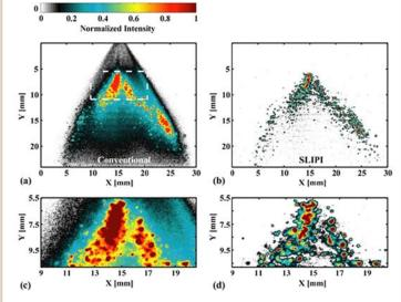
Images of sprays used, for example, in diesel engines, taken with conventional laser photography (a) and with SLIPI (b), which removes unwanted signals, such as the dark area surrounding the droplets in the left-hand figure.
