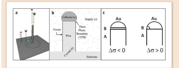
Nanowires are typically about 1-2 micrometres (µm) long and about 20-200 nm in diameter. They usually consist of two elements from groups III and V in the periodic table, but there are examples of combinations of elements from groups II and VI, alloys of three or four elements, or only group IV elements. Gold is often used as the catalyst for growing nanowires.
