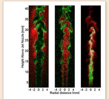
This figure shows LIF measurements of OH (warm product), CH (flame edge), CH<sub>2</sub>O (cool zone) and traces of uncombusted fuel (cold zone) in a turbulent jet flame. Each image contains two products. Left: OH (red) and CH (green), Middle: CH<sub>2</sub>O (red) and CH (green), Right: CH2O (red) and fuel (green).
