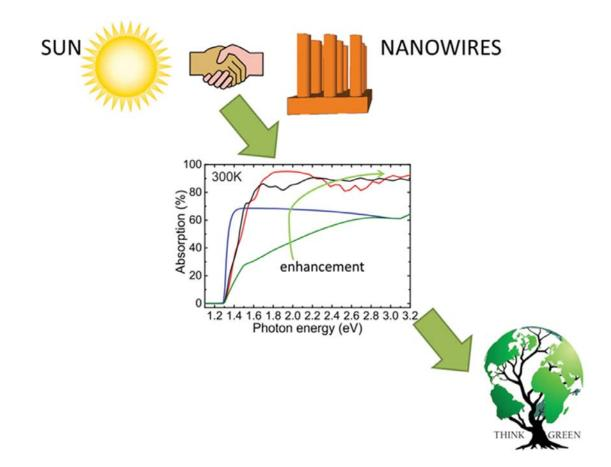
The diagram suggests how improved absorption of sunlight through nanowires is a promising route to generate more green energy. The absorption spectra have been adapted from Paper V. The green, blue, red and black traces, demonstrate the absorption of different photon energies (colors of sun light) by an indium phosphide (InP) thin film of 167 nm thickness, an InP thin film of 2 µm thickness, an InP nanowire array at normal incidence, and an InP nanowire array at 45° incidence respectively.
