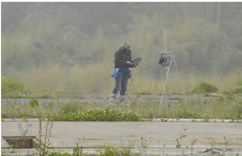
Figure 5. PTV measurements close to the fence of the Fukushima Daiichi reactor site in 2013 using a thin steel frame to cause minimal obstruction of the ^{134}\text{Cs} , ^{137}\text{Cs} photon field.
