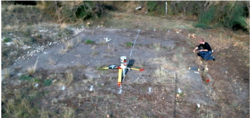
Figure 8. A Photograph of the PTV ratio measurement grid and radionuclide mapping of the radioactive waste (Radon type) repository. The grid was constructed with white markings on the ground in combination with a tape measure.
