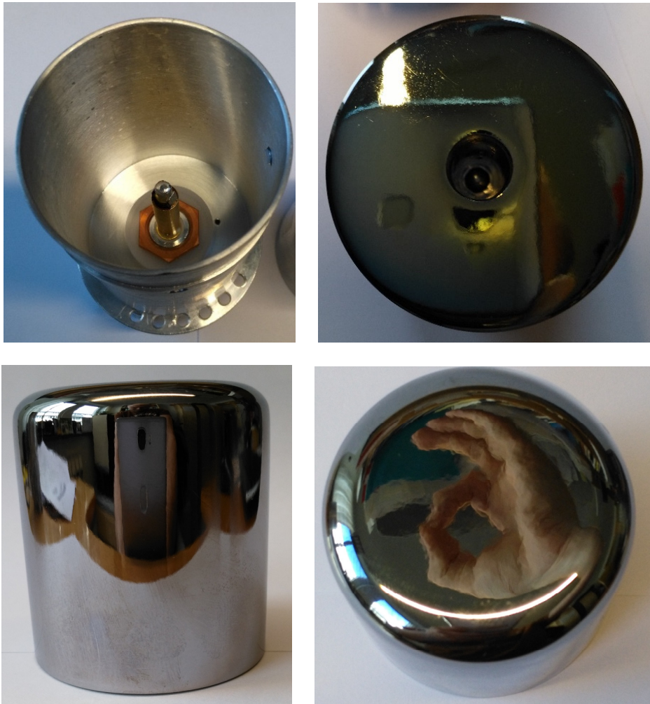
Figure 21. A photograph of the central electrode (upper left), the germanium crystal bottom (upper right), the bulletized top (lower left), and the detector front face (lower right) of a disassembled 22% (rel. efficiency) ORTEC n-type PopTop™ detector. The near perfect crystal structure surface and outer thin ( 0.6\ \mu\text{m} ) contact presents a mirror-like surface.
