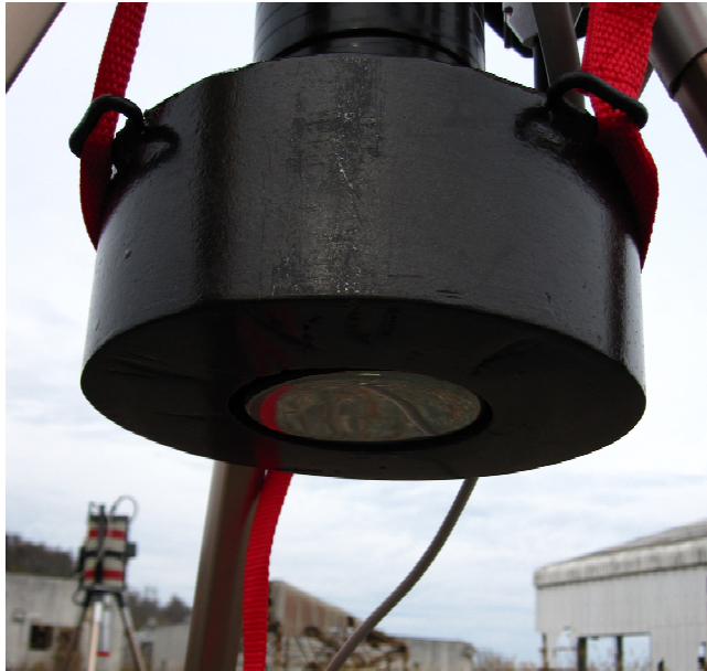
Figure 13. The collimator used in Paper IV applied to the detector, limiting the field of view to a radius of approximately 6 m.
