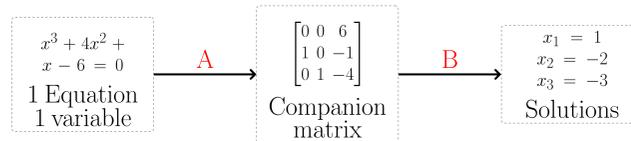
A. Copy polynomial coefficients into the companion matrix. B. The eigenvalues of the companion matrix are the solutions.
