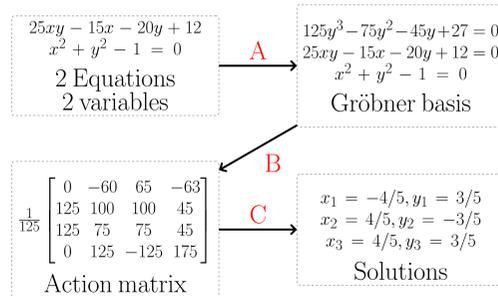
A. Generalized gaussian elimination. B. Copy elements from the Gröbner basis to form a generalized companion matrix. C. The eigenvalues and eigenvectors of the action matrix yield the solutions.
