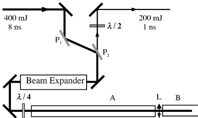
FIG. 3. Stimulated Brillouin scattering (SBS) compressor.  $\lambda/2$  (half-wave) and  $\lambda/4$  (quarter-wave) retarding plates are inserted.  $P_1$  and  $P_2$  are plate polarizers placed at the Brewster angle,  $L$  is a lens of 15 cm focal length,  $A$  is a 150 cm and  $B$  a 30 cm glass tube with pure water.
