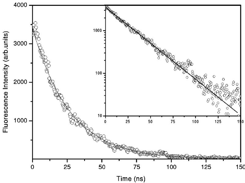
FIG. 4. Typical experimental curve (dots) from the  $7s\ 3S_1$  state of Cd I, with an exponential fit (solid line) that gives a lifetime of 24.4 ns. The inset shows the same data in a semilogarithmic representation.
