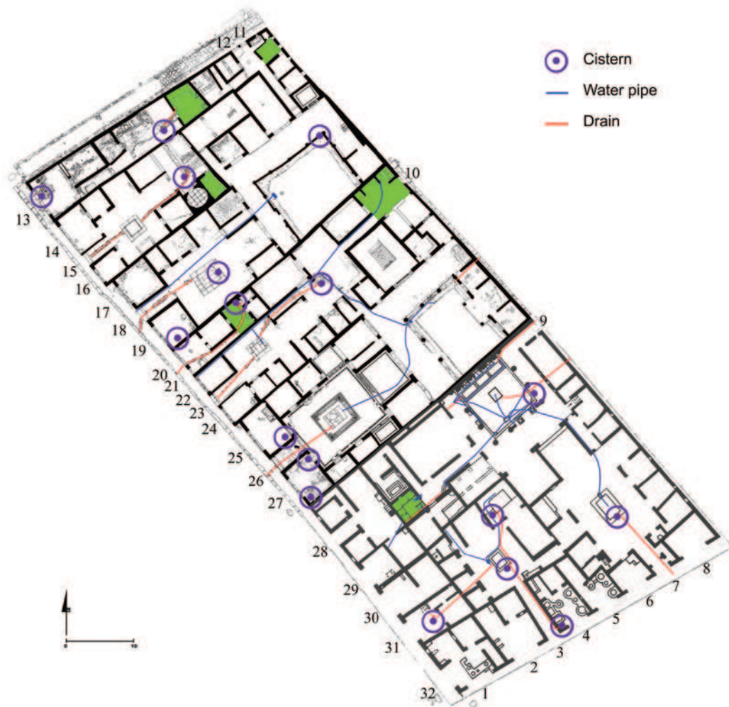
Fig. 14. Water pipes and cisterns in insula V 1. Blue lines used for inlets, red for drains; kitchen areas in green. By Henrik Boman.
