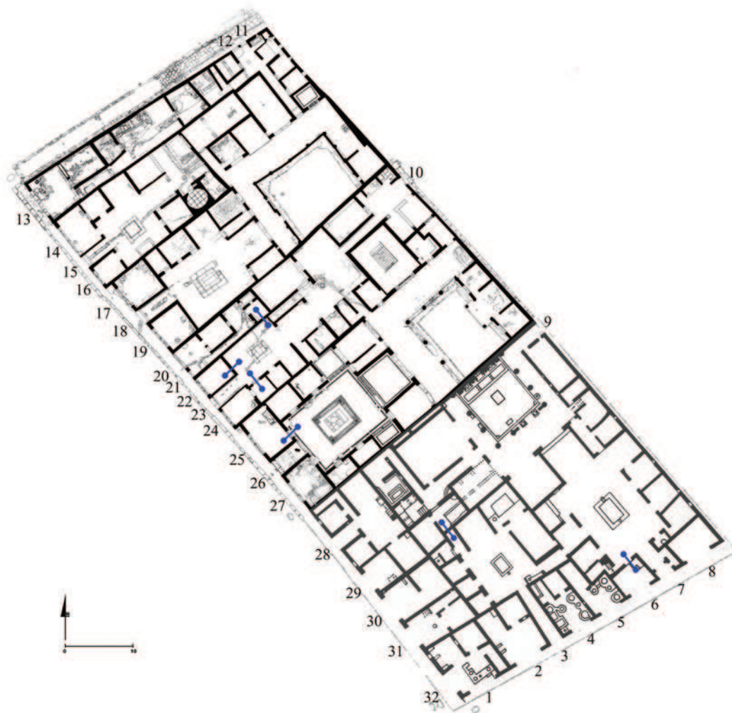
Fig. 36. Plan of the double atrium house of Caecilius Iucundus and taberna V 1,20–21, with indications for doors that were walled up in antiquity and the position of the cesspit and down-drain of the second-storey latrine. By Ezequiel Pinto Guillaume & Henrik Boman.
