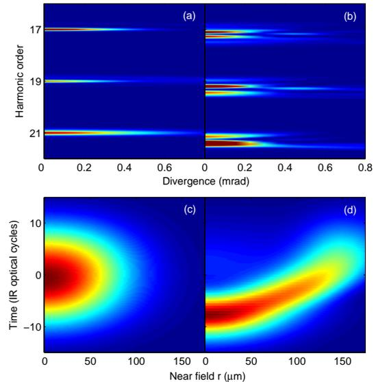
FIG. 9: Calculated far field spatial profile of different harmonic for two different peak intensities,  $1 \times 10^{14}$  W/cm<sup>2</sup> (a) and  $3.3 \times 10^{14}$  W/cm<sup>2</sup> (b). Spatio-temporal distribution of corresponding fundamental beam at the exit of the medium (c) and (d).
