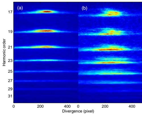
FIG. 8: Harmonic spectra at two different intensities, measured to be  $2 \times 10^{14}$  W/cm<sup>2</sup> (a) and  $\sim 5 \times 10^{14}$  W/cm<sup>2</sup> (b). A 21 mm gas cell was used and the focus point of the infrared beam was in the middle of the cell. Note the significant blue shift of the spectral distribution at high intensity.
