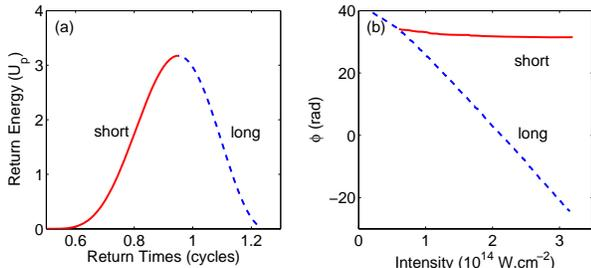
FIG. 1: (a) Classical calculation of the kinetic energy of the electron as a function of the return time. (b) Calculation of the intensity dependence of the 19<sup>th</sup> harmonic phase for the short and long trajectories using the strong field approximation [19].
