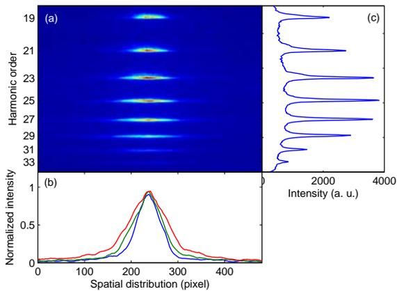
FIG. 4: (a) Experimental measurement using a 21 mm Ar gas cell and a fundamental intensity of  $I = 10^{14}$  W/cm<sup>2</sup>; (b) Spatial profile of the 19<sup>th</sup> (blue), 23<sup>rd</sup> (green) and 27<sup>th</sup> (red) harmonic (c) Spatially integrated spectrum.
