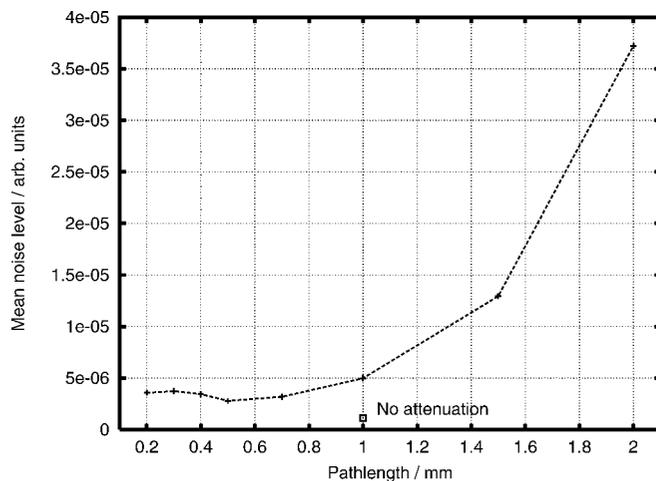
FIG. 9. Mean noise level in the spectral region  $4500\text{--}4250\text{ cm}^{-1}$  as a function of pathlength calculated from Fig. 8. Source was attenuated for data points connected with lines. The source was not attenuated for the isolated data point (box) at a pathlength of 1 mm.
