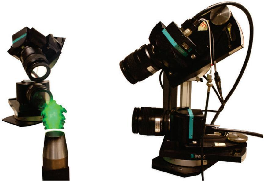
Figure 6.9 The camera arrangement used for measurements in vertically oriented volumes above the burner. The height of the measurement volume was ~50 mm. (Photo and editing A. & A. Petersson.)
