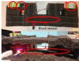
Figure 2. Flex charging massager prototype (1 active indicator, 2 vibrator, 3 charge indicator)
