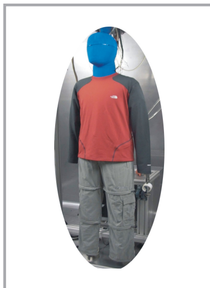
Figure 2. Fabric sweating thermal manikin “Walter”.
