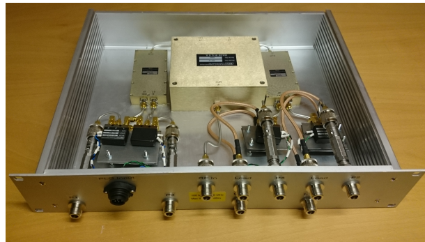
Figure 29: The feeding network mounted in a standard 19" rack case. Note that half of the switches are not visible since they are shielded by sheets of mu-metal.
