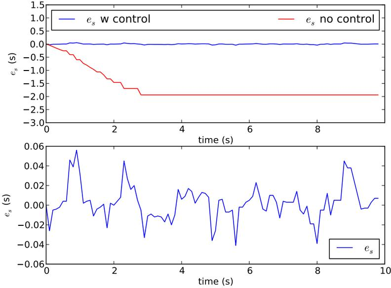
**Figure 7.10** Sync error compared with (blue) and without (red) control. In the uncontrolled case, the encoding pipeline stalls which is why the encoding error seems to remain constant after 2.5 seconds. The lower plot shows the sync error from the upper plot in detail.
