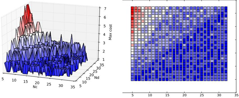
**Figure 8.11** The worst case individual costs (non-normalized) for scenarios of various sizes, all using *trade timeout* of 10 which has experimentally been proven sufficient for all the cases in this simulation to reach their lowest costs.  $w_l$  is set to 1 (i.e., the cost is the same as the number of repository accesses), with the plot shown both from the side and from above to make the cost breakpoints more visible.
