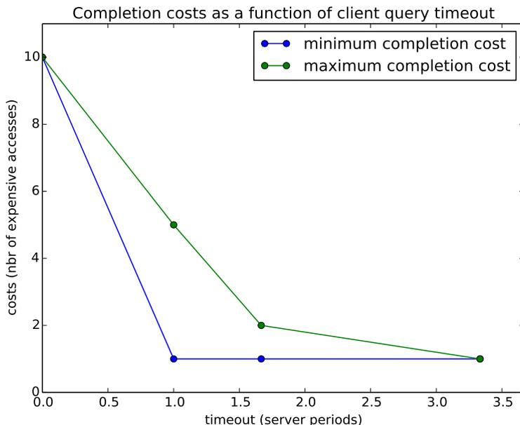
**Figure 8.26** The maximum and minimum costs for a client to complete its data set as a function of the *query timeout* setting. For high timeout values the performance is consistent while for lower values it starts to fluctuate. A timeout of 0 means that the client always performs a default action.
