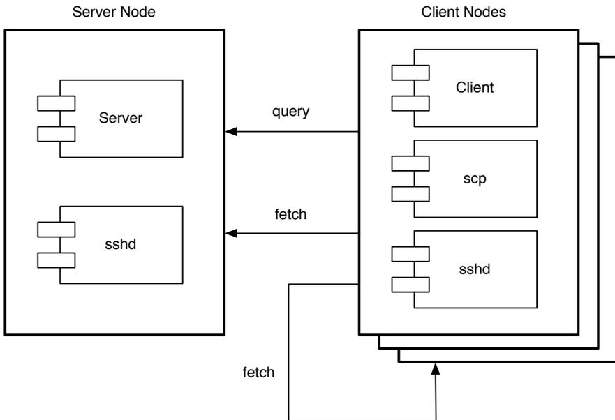
**Figure 8.18** Component diagram showing the two node types and their software components. The Server and Client components are written in Python, while the sshd and scp components are part of the OpenSSH software distribution[OpenSSH, 2014].
