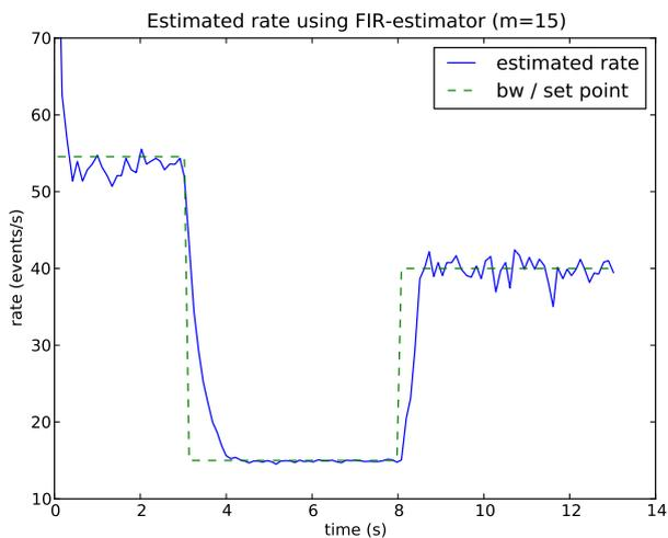
Figure 6.9 Estimation and control using event window
