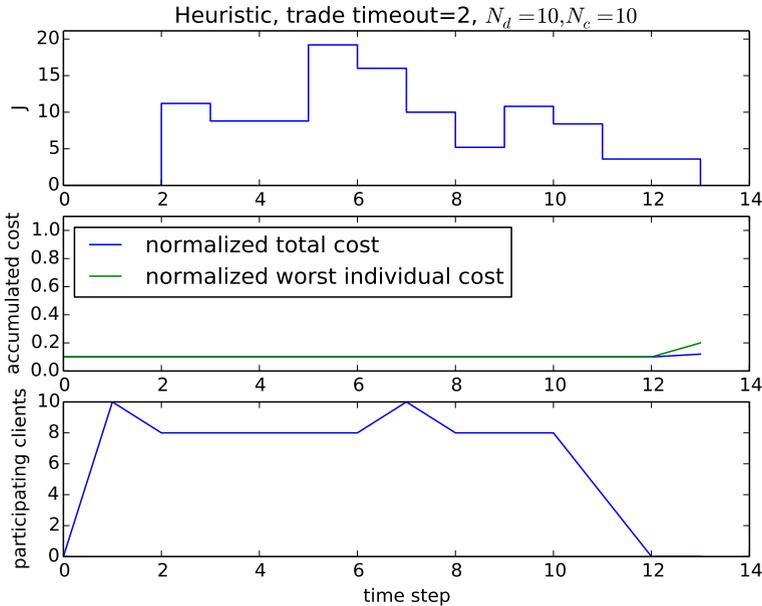
**Figure 8.10** System trajectories for the example in Section 8.6, with the *trade timeout* parameter set to 2, resulting in lower individual and total costs at the expense of more time steps. Only a single client is forced to do two repository accesses, which is seen in the slight increase of worst case cost in the final time step. Without normalization, the accumulated total cost is 12, the average cost is 1.2 and the worst case cost is 2.
