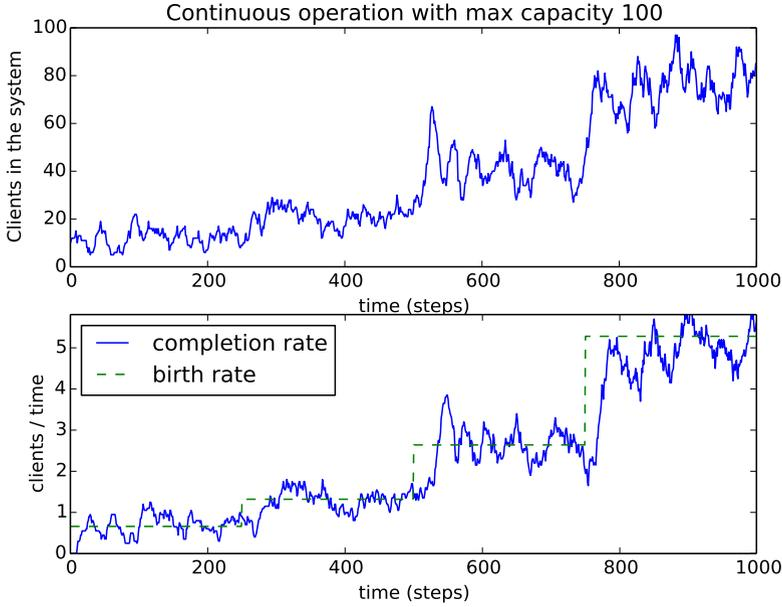
**Figure 8.16** Simulation of an exchange system with  $N_d = 16$  in continuous operation with new clients arriving through a Poisson process with increasing birth intensity. The system remains uncongested as intensity goes well above 3. The completion rate is calculated over a 20 time steps long sliding time window.
