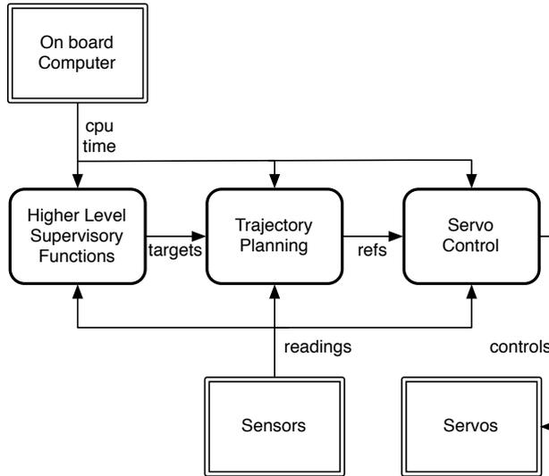
**Figure 2.2** A schematic over a simple mobile robot system. The square blocks represent hardware functions that require power, the round-corner shapes are software functions that require cpu-time to run. The complex dependency situation makes it non-trivial to determine how to prioritize in a situation with insufficient resources to run the system at nominal performance.
