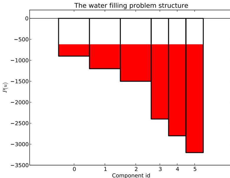
**Figure 6.1** The structure of the water filling problem. The geometry of the "tubes" is defined by the cost function and the optimal solution is found as the water surface if the tubes are filled to a common level.
