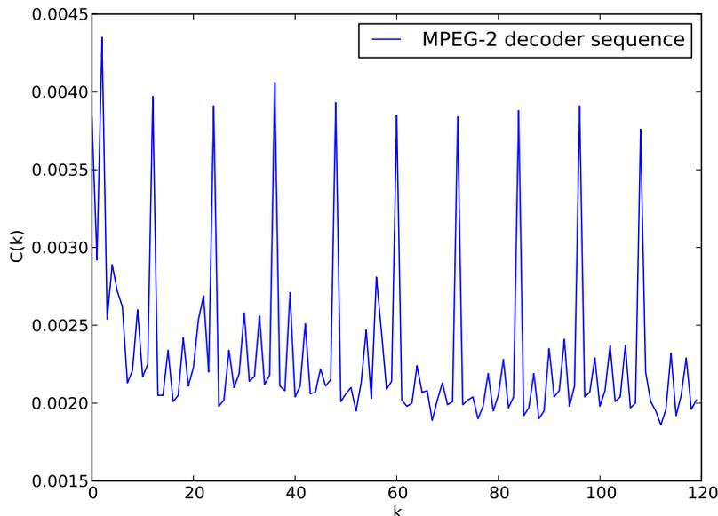
**Figure 7.6** A sequence of execution times for an MPEG-2 decoder working on a video stream. This encoding standard interleaves complete image descriptions with delta descriptions. Decoding a complete image is significantly harder, causing the high peaks.
