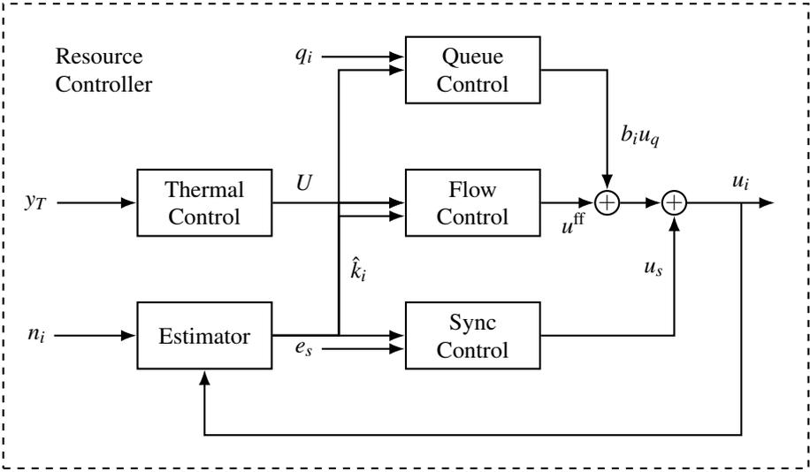
**Figure 7.4** The resulting control structure including estimation, feedforward flow control based on the estimated model parameters and the available CPU resource and feedback based on queue state and sync error.  $b_i$  refers to the coefficients in Equation (7.16).
