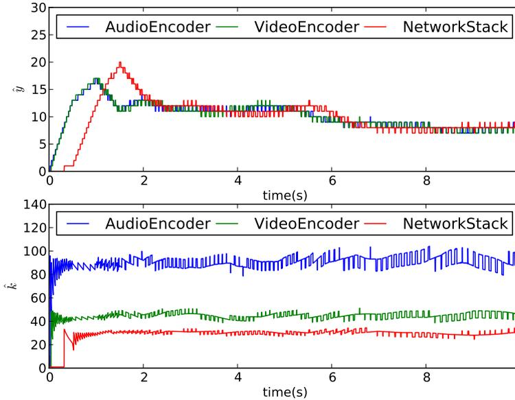
**Figure 7.8** Rate and parameter estimation for all three tasks. Rates are estimated by counting events with a sliding time window with length 1 second. The network stack (red) lags behind in the beginning due to queue control.
