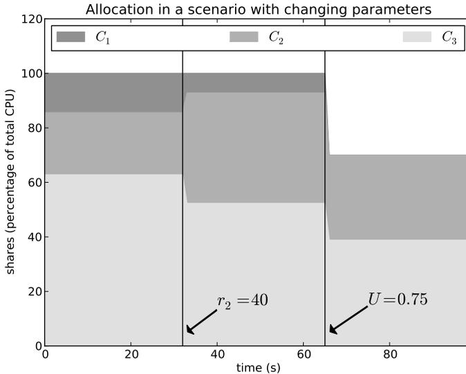
**Figure 6.4** A scenario where the problem parameters change over time, assuming allocation is computed every second. At 33 seconds,  $r_2$  changes to 40 and at 66 seconds, the total available resource level drops by 25%.
