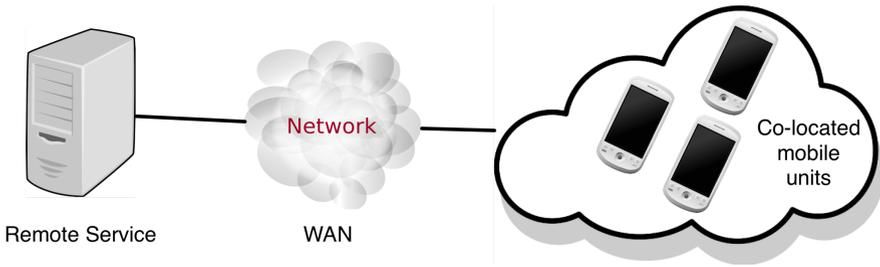
**Figure 2.3** The use of cloud computing services, such as remote data storage or media streaming, by mobile devices is very natural and in some cases even necessary in order to deal with limited built in storage and sandboxed applications. What has yet to happen is the inclusion of the mobile devices as part of the cloud in the form of service providers.
