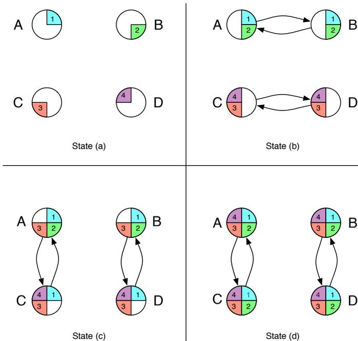
**Figure 8.7** A graphical representation of the state changes used in the *Empty initial state* example. The example uses 4 clients ( $\{A, B, C, D\}$ ) and 4 data objects ( $\{1, 2, 3, 4\}$ ). The arrows represent the trades that resulted in the current state.
