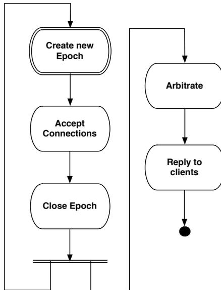
**Figure 8.19** A diagram of how the main decision server loop operates. The system starts by creating a new epoch, which then accepts new client queries until the timeout is reached and the epoch is closed. Immediately afterwards, a new epoch is created which accepts subsequent client connections, while the arbitration is carried out in parallel.
