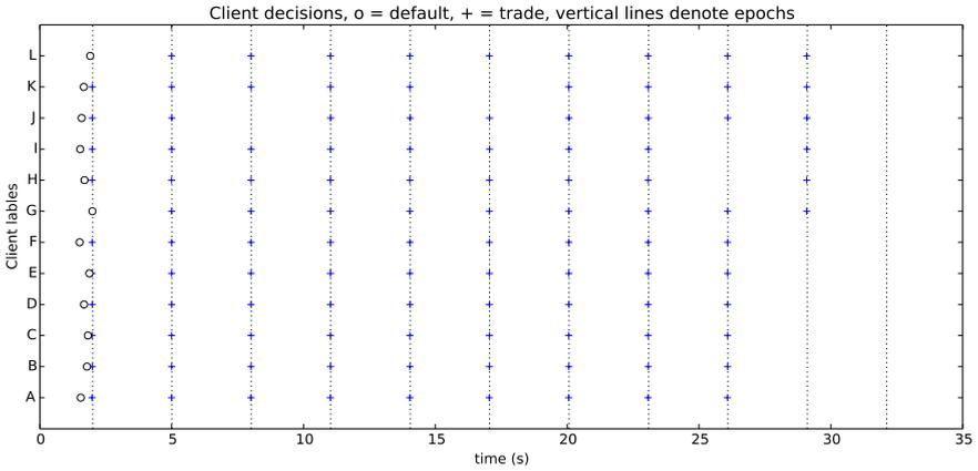
**Figure 8.23** A graphical representation of what actions the clients are taking over the course of the experiment for a case where the *query timeout* is 10 seconds. '+' denotes a trade while 'o' denotes a default action. The vertical lines show the epoch timeouts.
