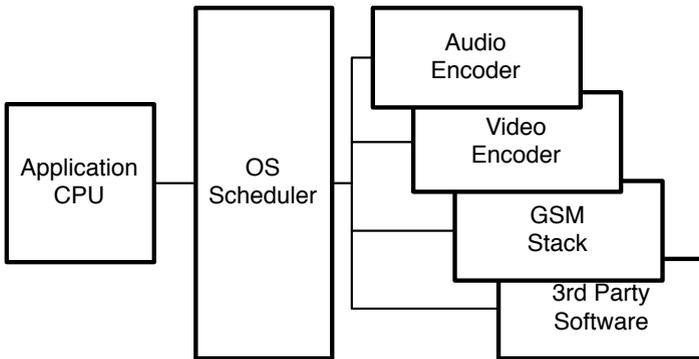
**Figure 5.1** A typical use case for a smart phone with support for 3rd party software. The application CPU is commonly a low power chip with limited precision running a fully featured OS such as the Linux-based Android platform.
