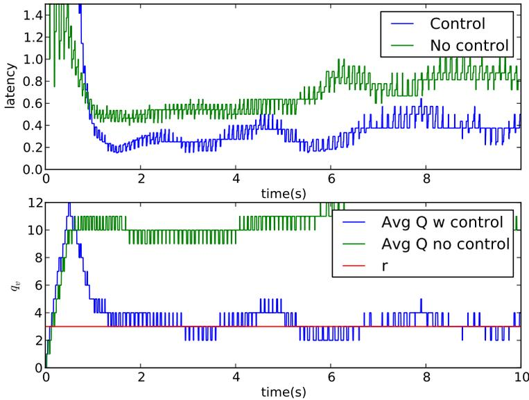
**Figure 7.9** End-to-end latency and average queue length compared with and without control. The uncontrolled case (green) is about 2-3 times worse than what it obtained through control (blue).
