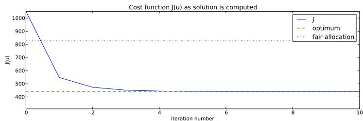
**Figure 6.3** A plot of how the cost function decreases in value for each iteration in the case illustrated in Figure 6.2, with the performance resulting from a fair allocation provided for comparison.
