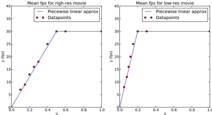
**Figure 5.4** Experimental results of controlling CPU-share for the MPlayer decoder using Linux 2.6.27 and Control Groups. The diagrams show how the frame rate per second (fps) depends on the amount of CPU share allocated to the decoder. The rate increases linearly with share until the movie can be played back at encoded rate.
