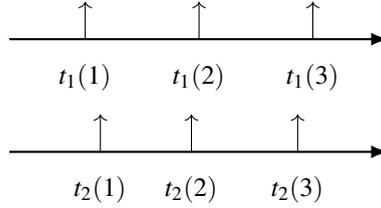
**Figure 7.2** Synchronization between two event sequences is one possible objective that can be solved using feedback resource management. The synchronization error,  $e_s(k) = t_1(k) - t_2(k)$ , is difficult to address using the feedforward strategy as this relies on collecting information over a number of events.
