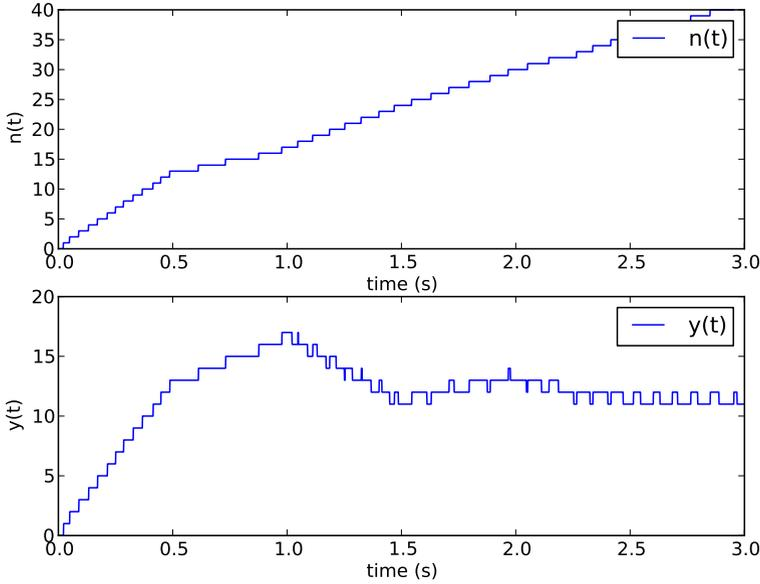
**Figure 5.3**  $n_i(t)$  and  $y_i(t)$  for one of the components in Chapter 7. Note that these are not sampled curves. Despite their jaggedness, both signals are defined for all  $t$ . Rate estimation is here done by a one second time window, i.e.,  $h = 1$ . Note that this will make  $y_i(t)$  lag behind by as much.
