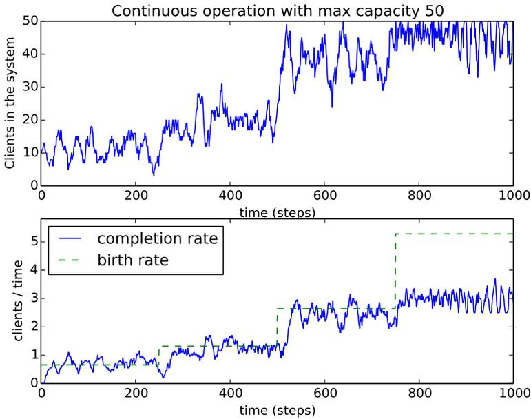
**Figure 8.15** Simulation of an exchange system with  $N_d = 16$  in continuous operation with new clients arriving through a Poisson process with increasing birth intensity. The system becomes congested when the intensity goes above 3. The completion rate is calculated over a 20 time steps long sliding time window.
