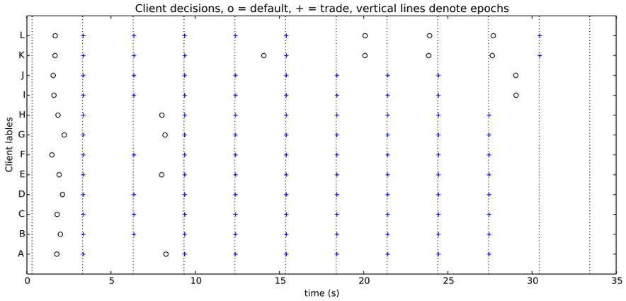
**Figure 8.25** A graphical representation of what actions the clients are taking over the course of the experiment for a case where the *query timeout* is 3 seconds. '+' denotes a trade while 'o' denotes a default action. The vertical lines show the epoch timeouts.
