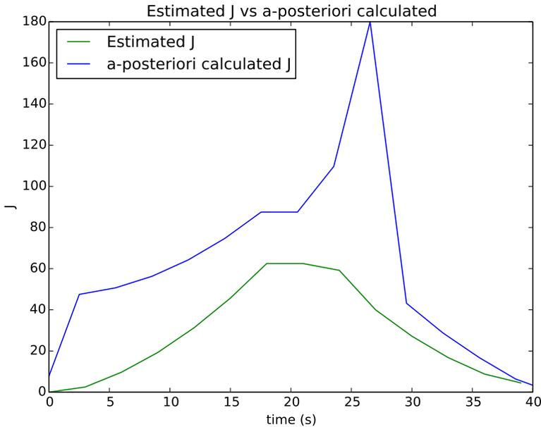
**Figure 8.22**  $J$  as a function of the server side system state estimate, sampled at the end of each epoch, compared to an a-posteriori calculated value based on the client side logs. Note how the estimate is always higher than the actual value, but the trend is generally the same.
