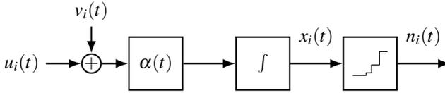
**Figure 5.2** A cyclic computation software component.  $u_i(t)$  is the CPU resource share assigned,  $v_i(t)$  is the disturbance on the assigned share caused by the environment,  $\alpha(t)$  is the execution speed of the CPU,  $x_i(t)$  is the accumulated execution, the last block is a staircase function mapping  $x_i(t)$  onto  $n_i(t)$ , which signifies the number of completed cycles.
