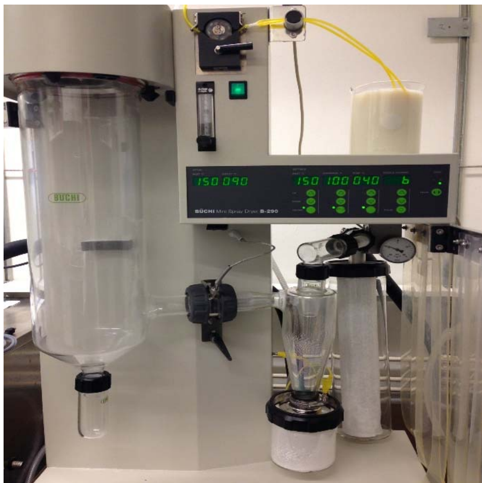
Figure 9. Lab-scale spray-dryer used in this work (Büchi mini spray-dryer B-290).
