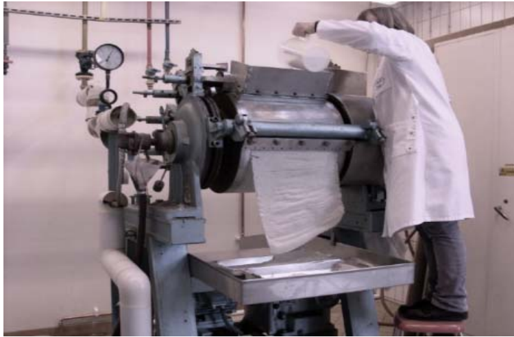
Figure 10. The drum-dryer used in the present work (Goudsche Machinefabriek) and the sheets of SMP. The average surface temperature of the drum was 115°C, and the drying duration was 40 s.
