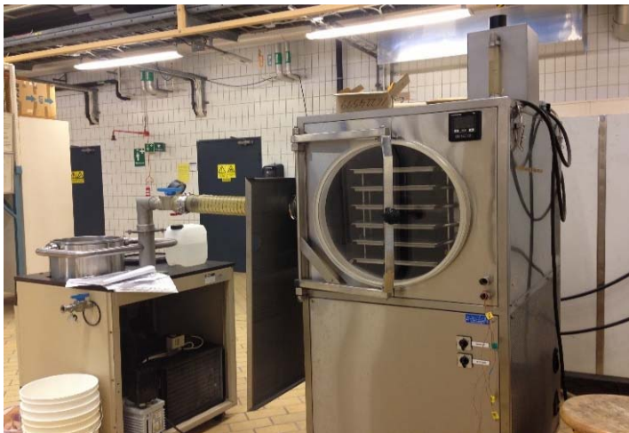
Figure 11. The freeze-dryer used (Labconco). The sample materials that had been frozen in metal containers were placed on the shelves inside the drying chamber.
