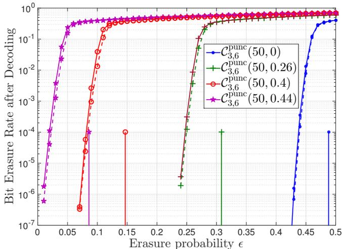
Fig. 11: BEC decoding performance and BP decoding thresholds of randomly punctured SC-LDPC codes. Solid lines represent results obtained with  $I_{\max} = 10$  and dashed lines represent results obtained with  $I_{\max} = 20$ .
