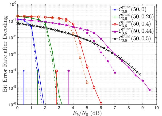
Fig. 12: BI-AWGNC decoding performance and predicted BP decoding thresholds of randomly punctured SC-LDPC codes. Solid lines represent results obtained with  $I_{\max} = 10$  and dashed lines represent results obtained with  $I_{\max} = 20$ .
