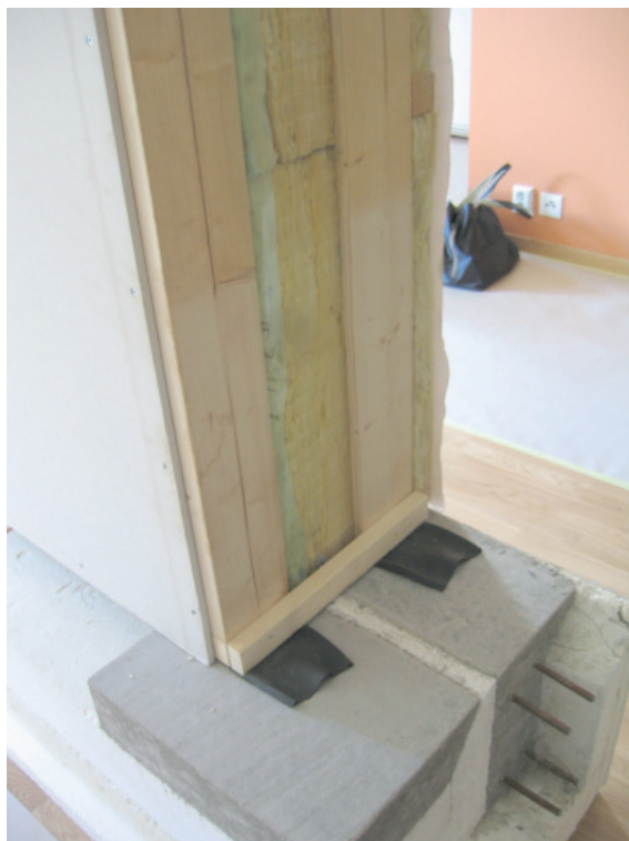
Figure 3.5 Model of wall and ground construction with the eps-insulation at bottom, the double concrete ground construction and the long side wooden wall.
