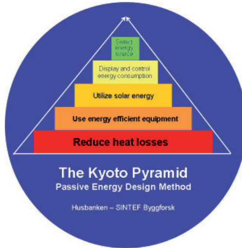
Figure 2.2 The “Kyoto pyramid” showing schematically the passive design principles (Husbanken/SINTEF Byggeforsk, Are Rødsgjøl/Tor Helge Dokka).
