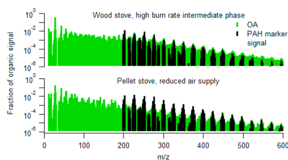
Figure 4. Normalized organic mass spectra from wood stove intermediate phase and artificially degraded, reduced air supply pellet combustion. The most abundant m/z is 28, tentatively attributed to CO^+ (see SI Figure S2). Note the logarithmic y-axes.
