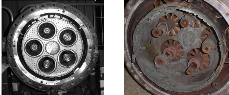
Figure 1.1 New burner assembly (left) and damaged by combustion instability (right) [3].
