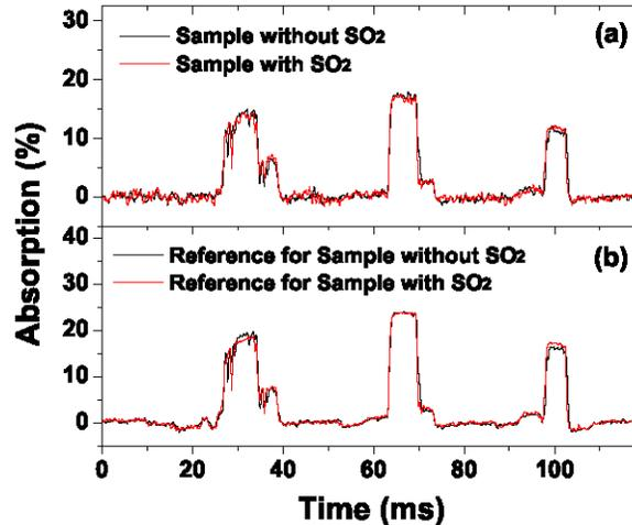
Fig. 8. (a) Sample absorption signals of mercury vapor with and without interference by SO<sub>2</sub> (2000 ppm, 10 cm) and (b) corresponding reference signals.
