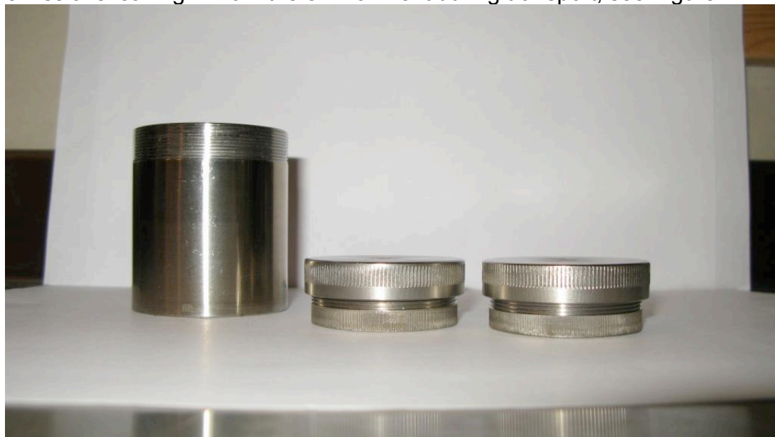
Figure 2. The bigger transport cup has Tenax in the bottom and can hold two PFS cups to avoid uptake of emissions during transport.
