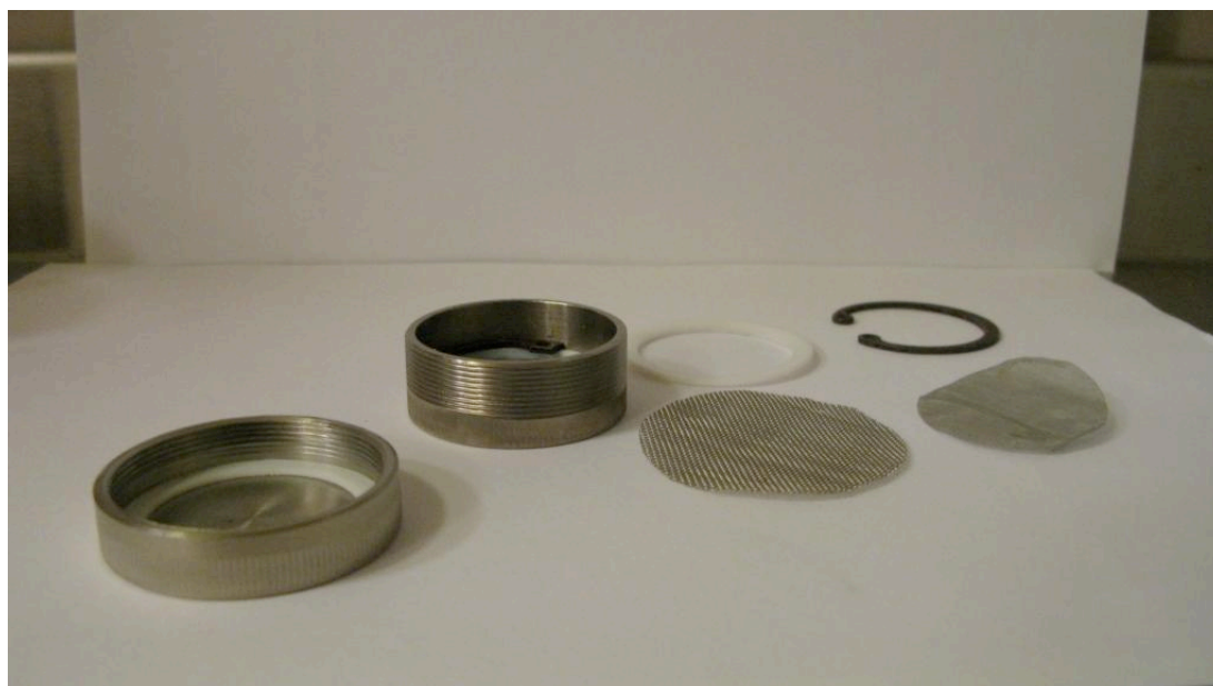
Figure 1. The PFS cup with assembly parts to hold the Tenax in place.
