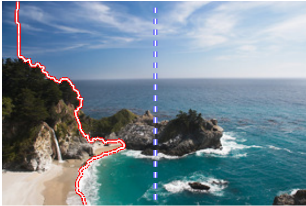
Figure 7.8: “Worst-case” test. The left and right side of the image is connected to the source and sink, respectively. The edge costs are determined by the image gradient. All flow must be communicated between the two computational threads when splitting the graph vertically.
