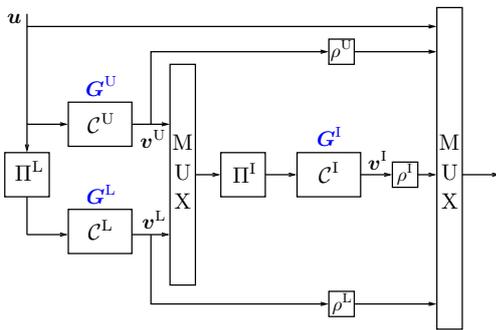
Fig. 3. Block diagram representation of an HCC encoder
