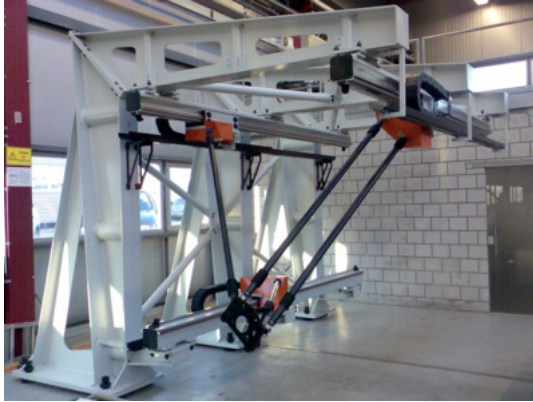
Figure 1.1 Gantry-Tau prototype developed within the SMErobot project.
