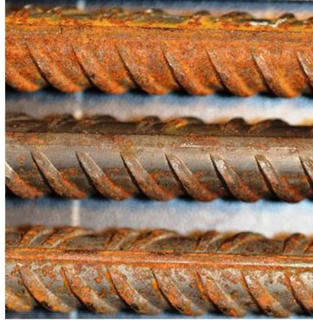
Figure 43. Photo of surface condition for an “as-received” steel bar.
