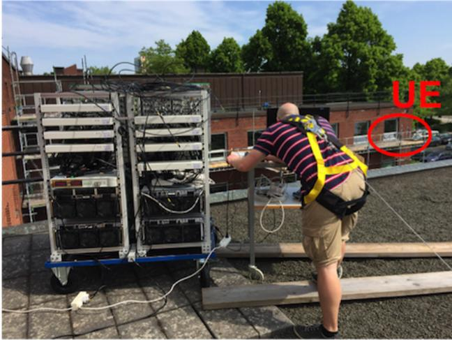
**Figure 14:** The outdoor test scenario setup with the BS deployed on the rooftop of the department building marked with two UEs on the opposite building wing.
