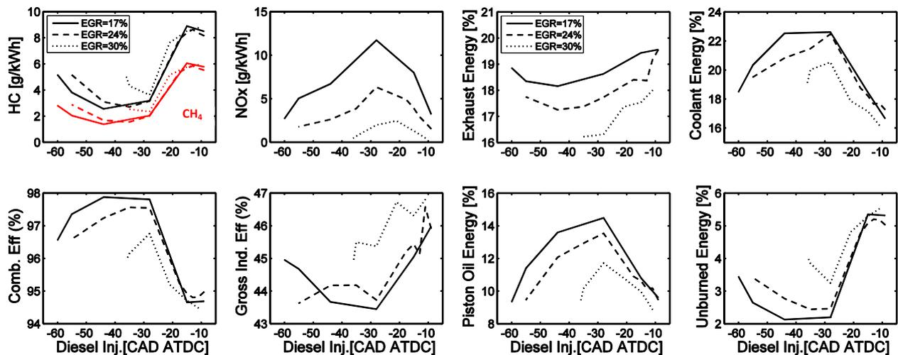
Figure 2: Emissions, efficiencies and energy balance for SR=70% transition from CDF towards RCCI combustion at different dilution levels
