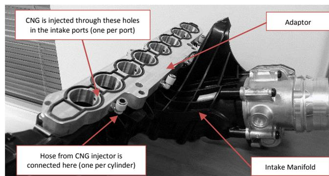
Figure 1: Adaptor plate for CNG injectors attached to intake manifold. Each injector supplies CNG to two different ports (one injector per cylinder)
