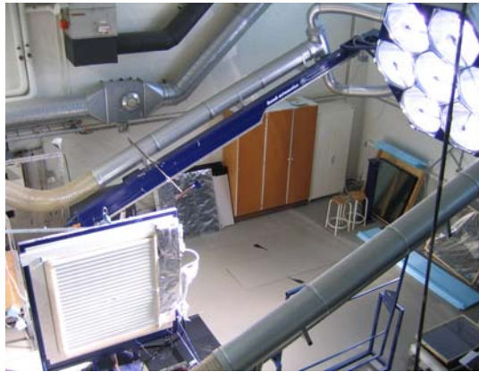
Fig. 4.2.1. The solar simulator with a mounted white aluminium shutter.
