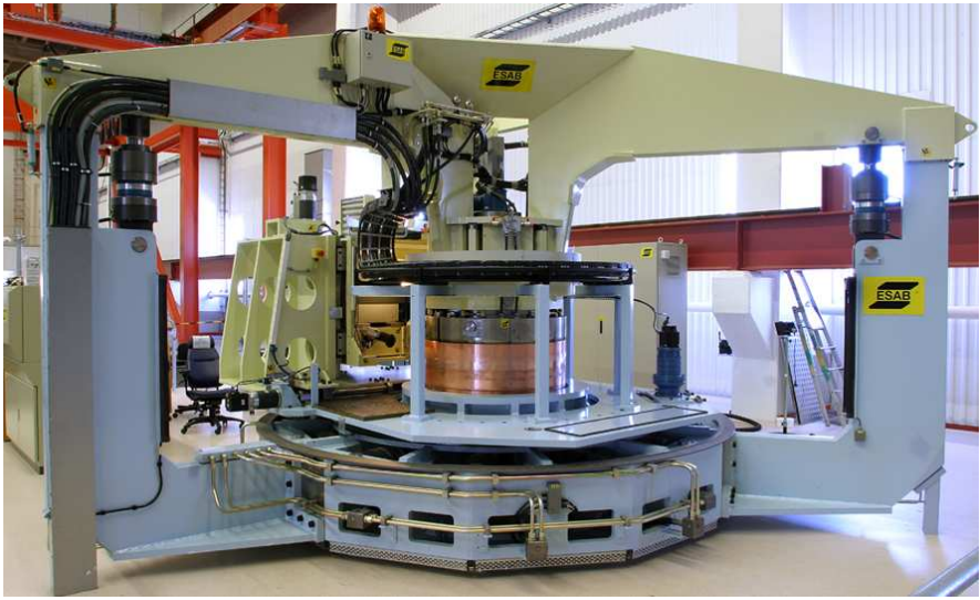
Figure 3. Purpose-built FSW machine for copper canister welding.
