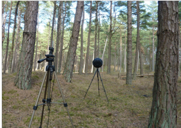
Picture 3. Measuring impulse response in pine forest.
