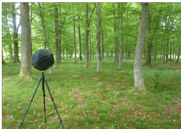
Picture 5. Measuring impulse response in beech forest.
