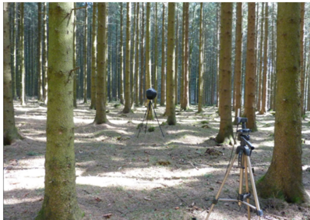
Picture 4. Measuring impulse response in fir forest.
