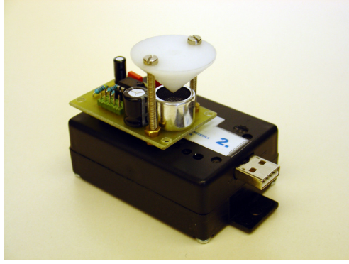
Figure 4 Stationary sensor network nodes with ultrasound receiver circuit. The nodes are packaged in a plastic box to reduce wear.
