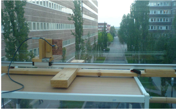
Figure 3.3: Linear positioning robot with TX probe antenna.
