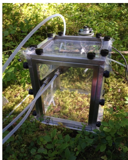
Figure 4. A soil chamber was placed on the frame with tap water filled in the channel to make the frame airtight.
